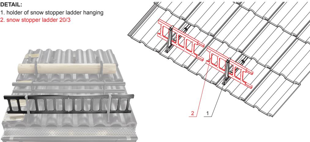
**MH** Galvanized steel prepainted – Copper brown – RAL 8004
